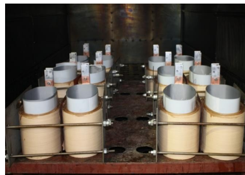
LV Insulation with resin impregnated cloth with class H glue , 3.5 hours 140C drying process
