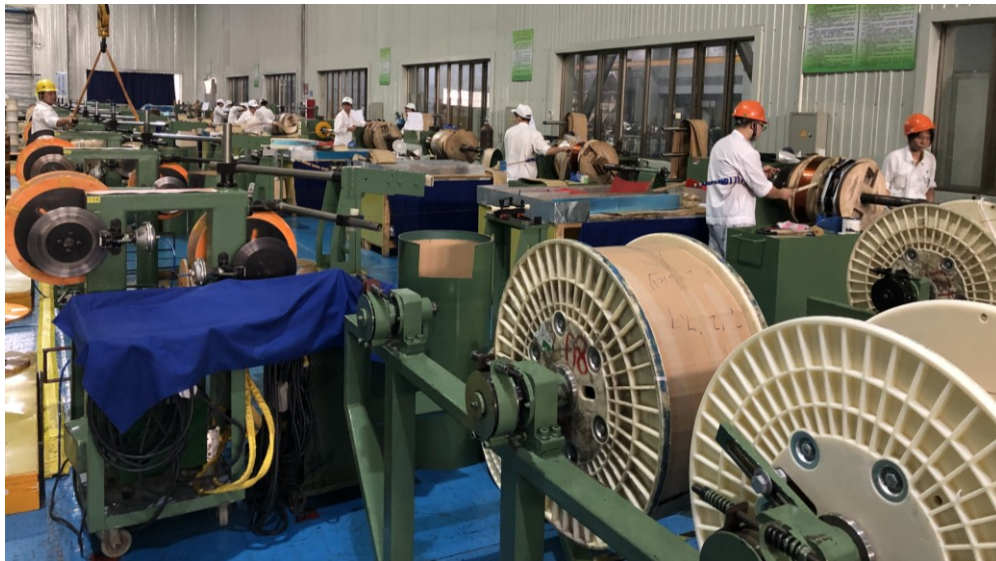
The continuous HV windings with extra two layers enforcing/sections with JSHP patented technique
